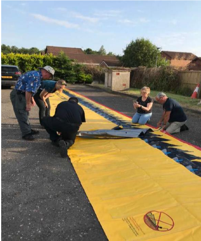
Testing of Watergate System by Local Flood Group (TIDECO) in Tillicoultry – 29 th June 2021
